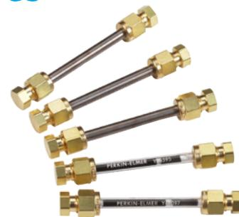
Fully conditioned Thermal Desorber tubes
