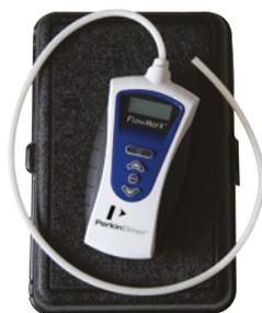
PerkinElmer's FlowMark™ flowmeter is specifically designed for use with gas chromatography (GC) instruments. The probe is applied directly to the gas flow stream and the measured flow rate is presented on the LCD screen.
