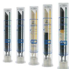
To meet the high flow needs of the LC/MS system, the hydrocarbon or moisture filled cartridges are positioned and placed in parallel. The incoming gas stream is split equally between the cartridges and the two streams are re-joined after purification but before the gas exits the base plate. Get up and running with speed and benefit from increased sensitivity by removing unwanted moisture and hydrocarbons. These filters typically last 3 to 6 months.
