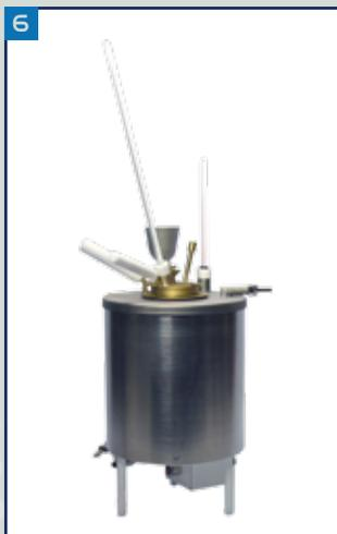
*The flash point of a flammable liquid is the lowest temperature at which it can form an ignitable mixture in air. A slightly higher temperature, the fire point, is defined as the temperature at which the vapour continues to burn for at least 5 seconds after being ignited.*
