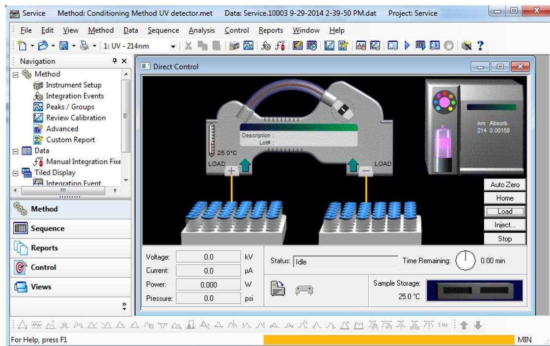
Click **Load** to move the trays to the front of the sample compartment. Inspect the interface block by using an angled mirror and penlight. Clean the interface block as required using the procedure in the *System Maintenance Guide*.
