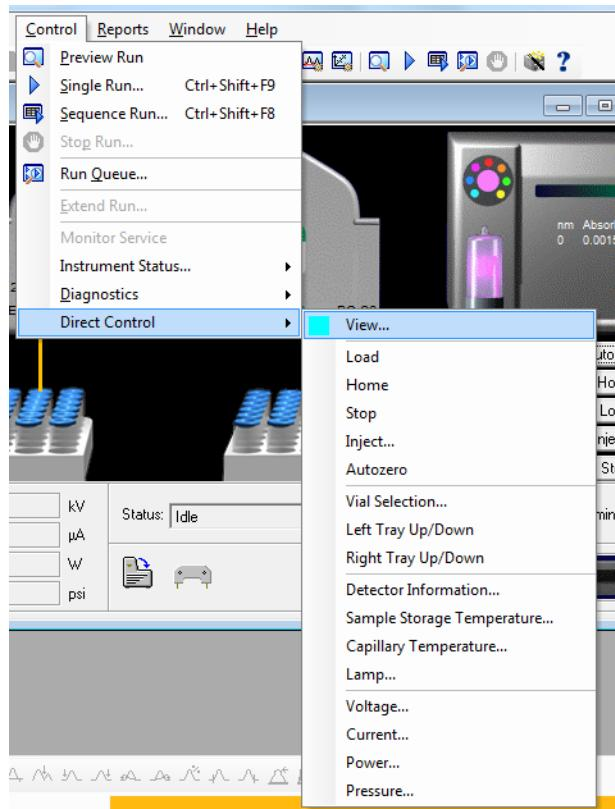
The **Direct Control** window allows manual control and reports the status of the instrument functions. Icons that confirm the status of the sample cover and cartridge are located in the lower part of the window ([Figure 5.8](#)). Verify the indicators show the sample cover closed and a cartridge installed. If the sample cover is open, or if no cartridge is installed, the trays cannot move.
